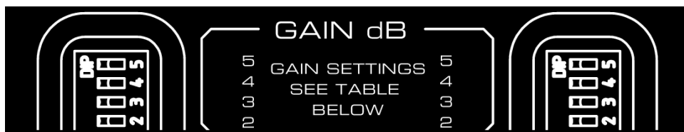
Figure 4: Left and right channel DIP switches for gain level settings
