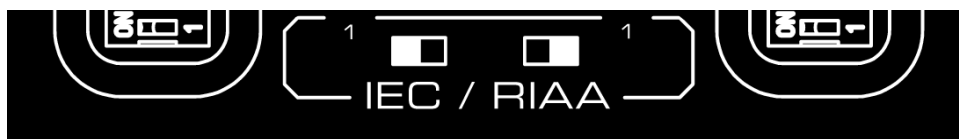
Figure 5: Left and right channel DIP switches for equalization curves
