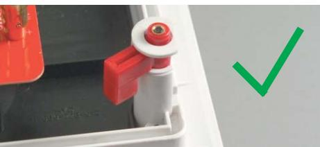
*Make sure that the red mounting tabs (6 per InWall system) do not stick out (photo above), but are in a position facing the inside (photo underneath) so that the InWall system will fit in the installation opening.*
