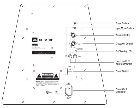
**Phase Switch:** This switch determines whether the subwoofer transducer's piston-like action moves in and out in phase with the main speakers. If the subwoofer were to play out of phase with the main speakers, the sound waves from the main speakers could partially cancel out the sound waves from the subwoofer, reducing bass performance and sonic impact. This phenomenon depends in part on the placement of all the speakers relative to the listening position and to each other in the room.
