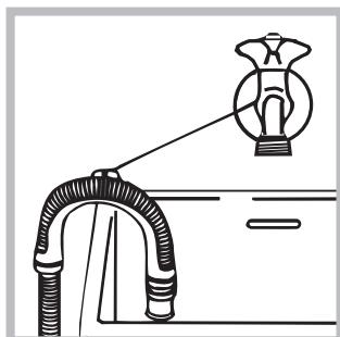
Alternatively, rest the drain hose on the side of a washbasin or bathtub, fastening the duct supplied to the tap (see figure).
