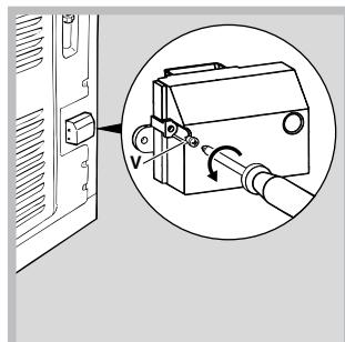
1. Loosen the screw V in the terminal board and pull the cover to open it (see figure).
