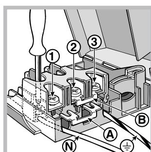
2. Position the connection supports A (see figure) according to the connection diagram shown above. The terminal board is designed for single-phase 230 V connection: terminals 1, 2 and 3 are connected
